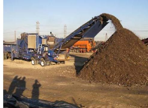
Fig. 7. “Plus 76-mm” waste is shredded.
