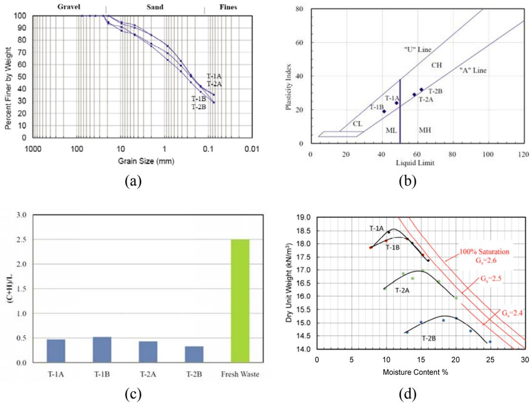
Fig. 5. Results of laboratory testing (minus 76-mm waste fraction): (a) grain-size distribution; (b) Atterberg limits; (c) (C+H)/L; and (d) modified Proctor compaction.
