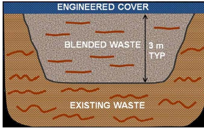
Fig. 1. Schematic of the intended final configuration of the existing and processed waste.
