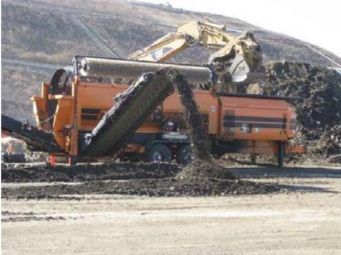
Fig. 6. Waste is screened by a trommel into “plus” and “minus” 76-mm particle stockpiles.
