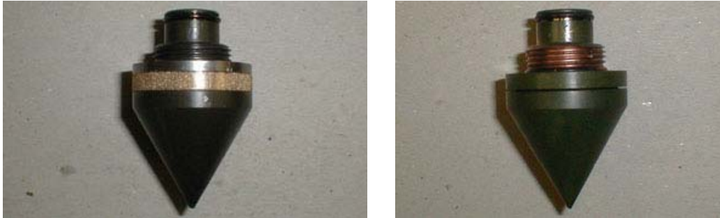
Figure 5: CPT tip with porous filter and slot filter respectively ( www.envi.se )
