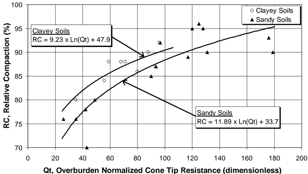
Figure 1. Correlation between Normalized Cone Tip Resistance and Relative Compaction estimated from in-situ density data
