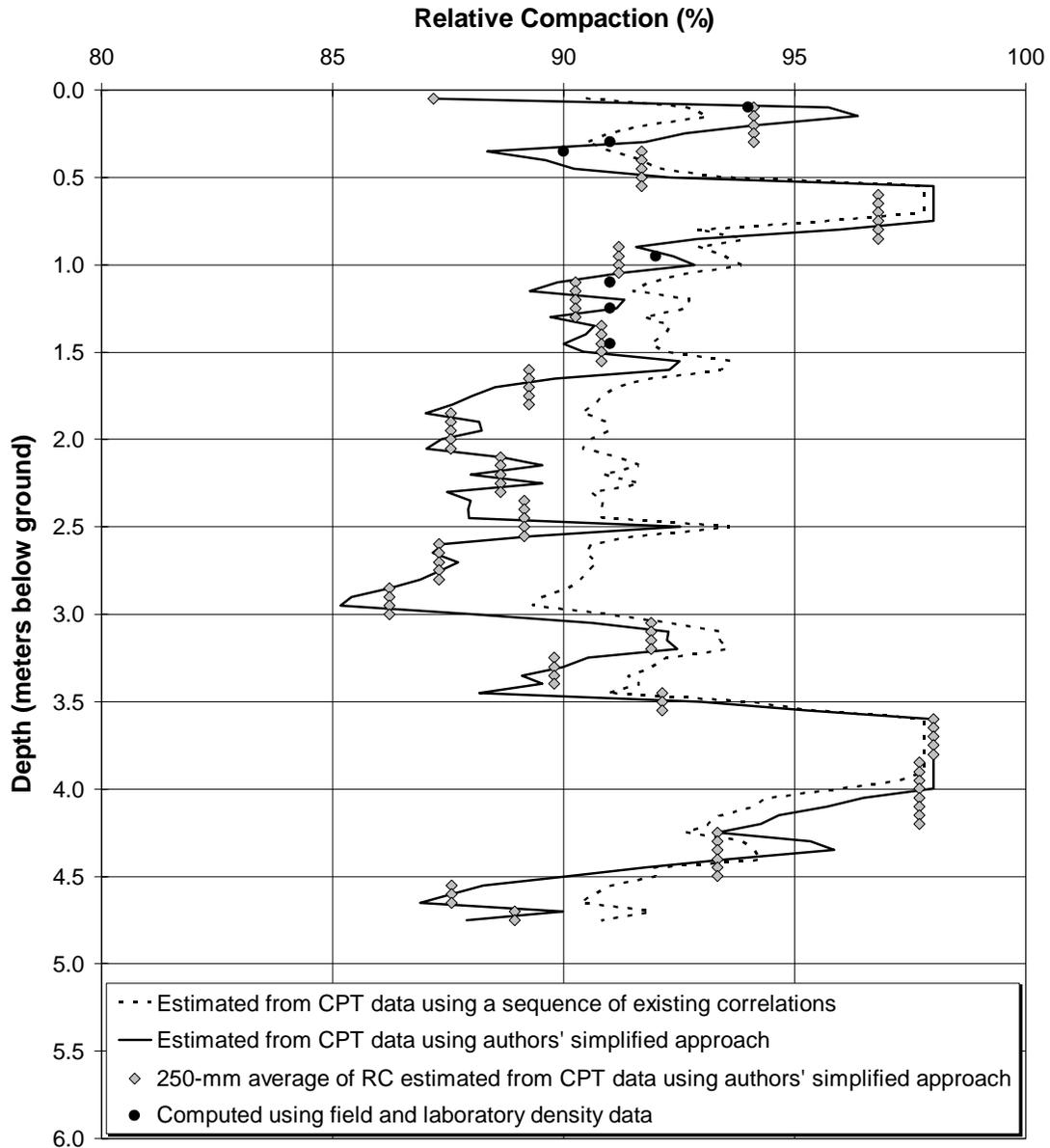
Figure 2. Typical log of relative compaction estimated from CPT Data and that obtained from conventional field testing
