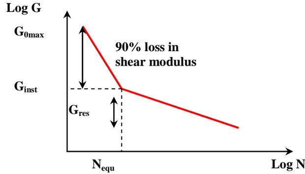
Figure1: Schematic representation of cyclic degradation of shear modulus in triaxial test
