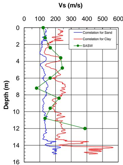
Figure 3: Comparison between measured  $V_s$  by SASW and by using CPT- $V_s$  correlating equations proposed by Andrus et al, 2003.
