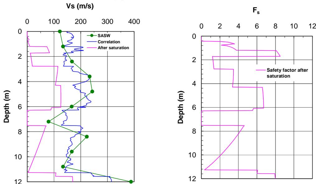
Figure 5:  $V_s$  profile in wetted conditions and safety factor against instability calculated using the proposed assessment method
