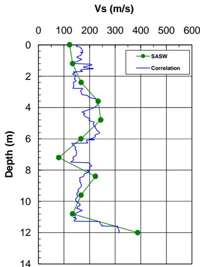
Figure 4: Calculated  $V_s$  profile in loess soil using a new CPT- $V_s$  correlation equation.
