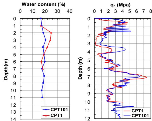
Figure 2: Water content and CPT profiles at initial conditions (CPT101) and after wetting (CPT1) (site Km 140, SNCF)
