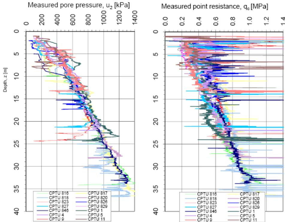
Figure 2. Variations in measured pore pressure (left), and cone resistance (right) in quick clay.
