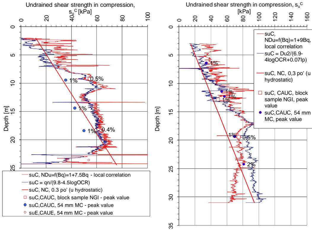
Figure 1. Interpreted  $s_u^c$  in borehole 823 (quick clay) to the left and borehole 809 (silt and clay at larger depths) to the right.
