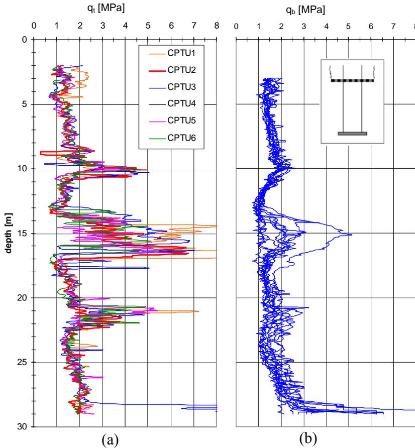
Figure 5. (a) CPT tip resistance data and (b) records of jacking force during pile installation.
