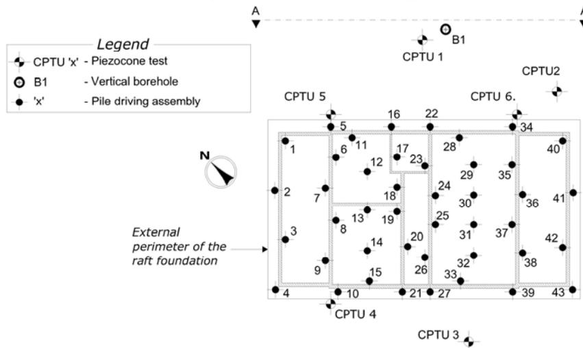
Figure 3. Plan of the building with piles lay-out and location of geotechnical investigations.
