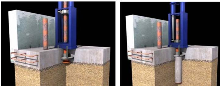
Figure 2. Pile installation process.
