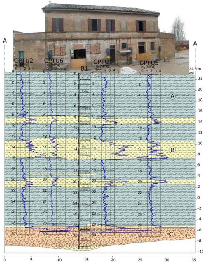
Figure 4. Schematic section (A-A in Figure 3) of the subsoil, from the in-situ testing logs and view of the building.
