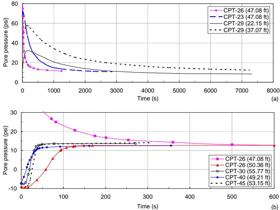
Figure 7. Pore pressures versus times for selected dissipation tests. (Note: result of CPT-26 at 47.08 ft is plotted in both Figures 7(a) and 7(b) for comparison. 1 psi = 6.89 kPa.)
