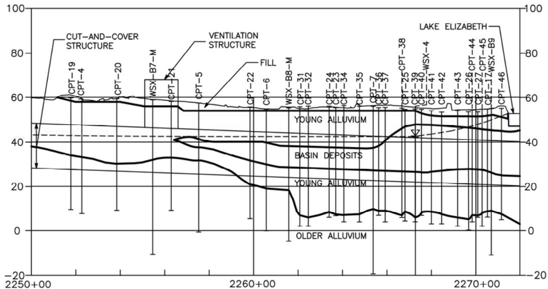
Figure 3. Inferred geologic profile near north of the lake updated with Phases 2 and 3 CPT investigations. (Note: vertical axis is elevation in feet and horizontal axis is station number in feet)
