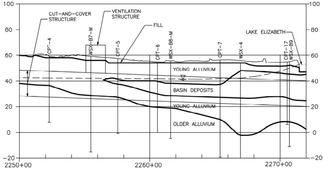
Figure 2. Inferred geologic profile near north of the lake based on borings and Phase 1 CPT investigation. (Note: vertical axis is elevation in feet and horizontal axis is station number in feet)
