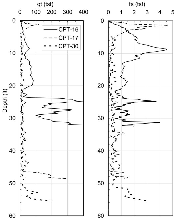
Figure 5. Logs of selected CPT soundings
