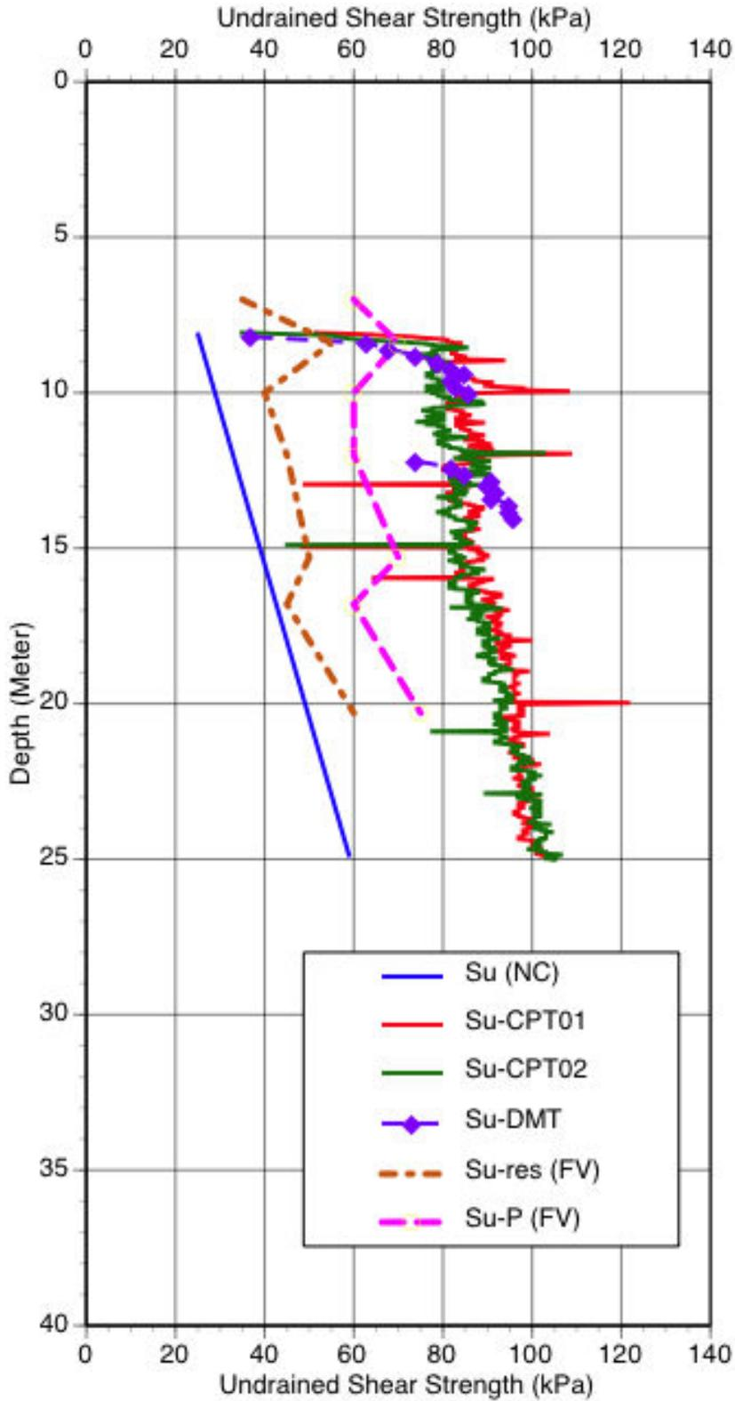
Figure 4: Undrained shear strength for site 2 obtained from DMT and CPTU with factor  $N_k = 11$  for CPTU calibrated on DMT and compared to undrained shear strength obtained from field vanes during the site investigation in 1966 for existing plant.
