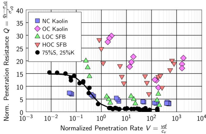
Figure 2. Effect of normalized penetration rate on normalized penetration resistance in five soils. (75% sand, 25% kaolin mixture; lightly and heavily overconsolidated silica flour-bentonite (SFB), and normally consolidated and overconsolidated kaolin data from Schneider et al. 2007).
