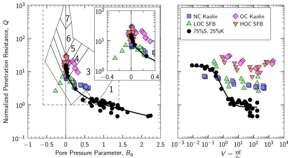
Figure 5. Effect of normalized penetration rate on the use of soil classification charts in five soils with corresponding normalized velocity and normalized penetration resistance plot (75% sand, 25% kaolin mixture; lightly and heavily overconsolidated silica flour-bentonite (SFB), and normally consolidated and overconsolidated kaolin data from Schneider et al. 2007).
