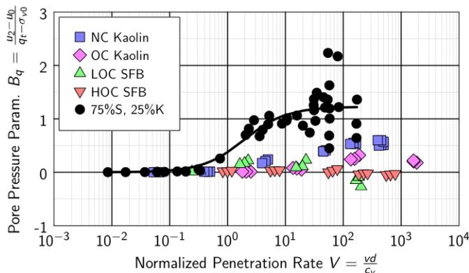
Figure 3. Effect of normalized penetration rate on the pore pressure parameter  $B_q$  in five soils. (75% sand, 25% kaolin mixture; lightly and heavily overconsolidated silica flour-bentonite (SFB), and normally consolidated and overconsolidated kaolin data from Schneider et al. 2007).
