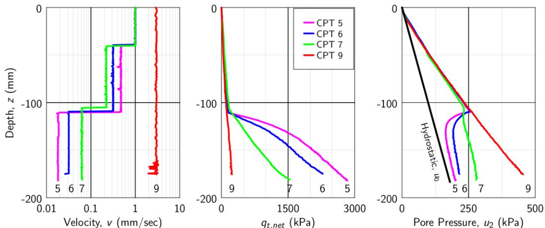
Figure 1: Variable penetration rate cone penetration testing profiles in 75% sand, 25% kaolin mixture.
