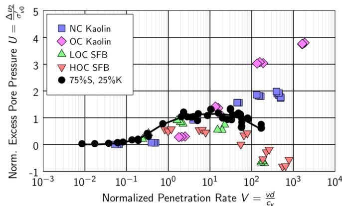
Figure 4. Effect of normalized penetration rate on pore pressure normalized by the initial vertical effective stress in five soils. (75% sand, 25% kaolin mixture; lightly and heavily overconsolidated silica flour-bentonite (SFB), and normally consolidated and overconsolidated kaolin data from Schneider et al. 2007).
