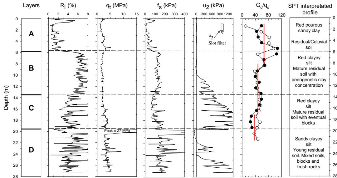
Figure 5: Piezocone test results for residual soils at the Campinas - Brazil site and interpretation of the main layers
