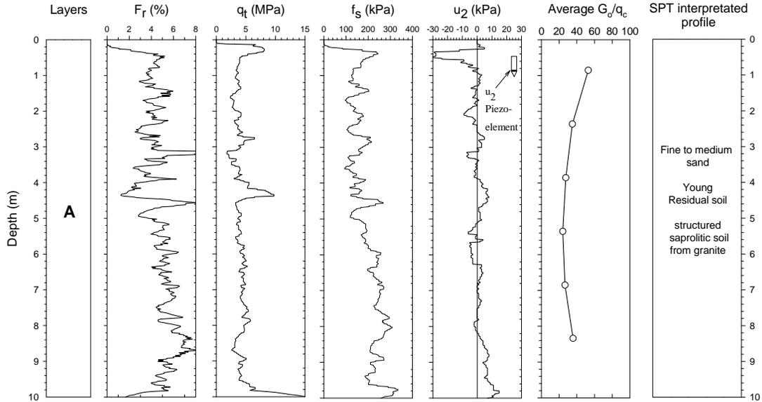
Figure 3: Piezocone test results for Porto ISC2 Site – Portugal residual soil
