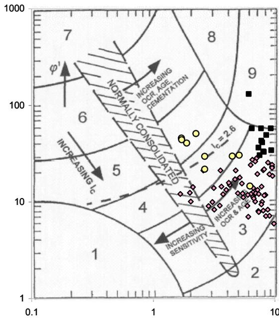
Figure 4. Q-F analysis for Location B (■: 0-3 m, ◇: 3-18m, ○: >18m)
