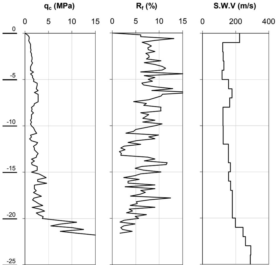
Figure 3. Mechanical CPT and SDHT results for Location B in Indonesia.
