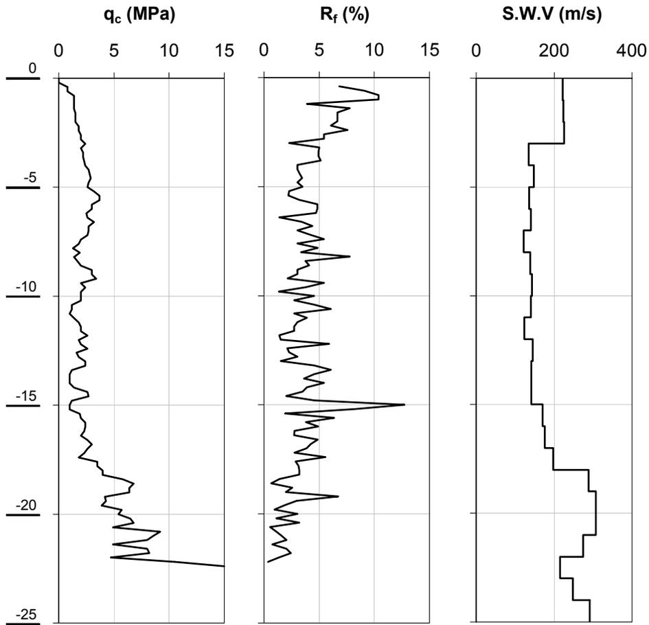
Figure 1. Mechanical CPT and SDHT results for Location A in Indonesia.
