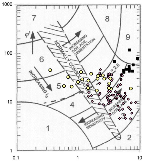
Figure 2. Q-F analysis for Location A (■: 0-3 m, ◇: 3-18m, ○: >18m)
