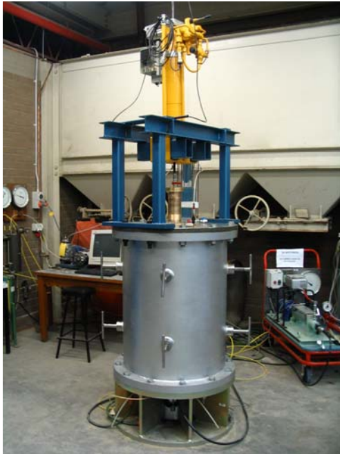
Figure 4. Penetrometer mounted on the top of the chamber
