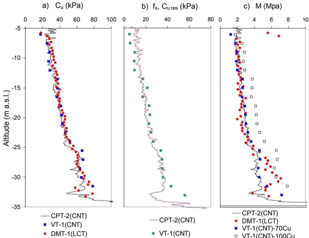
Figure 4. Strength and deformation characteristics of NC Neretva River clay based on CPTU, DMT and VT results: a) peak undrained shear strength; b) CPT friction sleeve vs. VT residual shear strength; c) modulus of compressibility.
