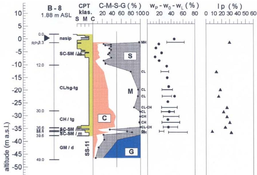
Figure 1. Typical soil profile at the BCT Ploce in Croatia.
