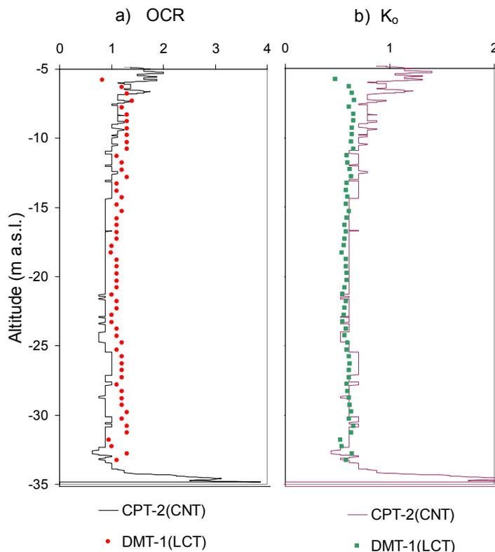
Figure 3. CPTU vs. DMT estimates of: a)  $OCR$  and b)  $K_0$ , in NC Neretva River clay, Croatia.
