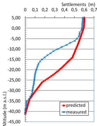
Figure 6. Comparison between measured and predicted settlement profiles.
