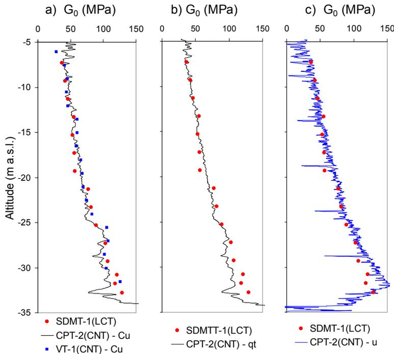
Figure 5. SDMT measured vs. estimated small strain shear modulus ( $G_0$ ) based on: a) undrained shear strength ( $C_u$ ); b) corrected total cone tip resistance ( $q_t$ ); c) excess pore pressure ( $\Delta u = u_2 - u_0$ ).
