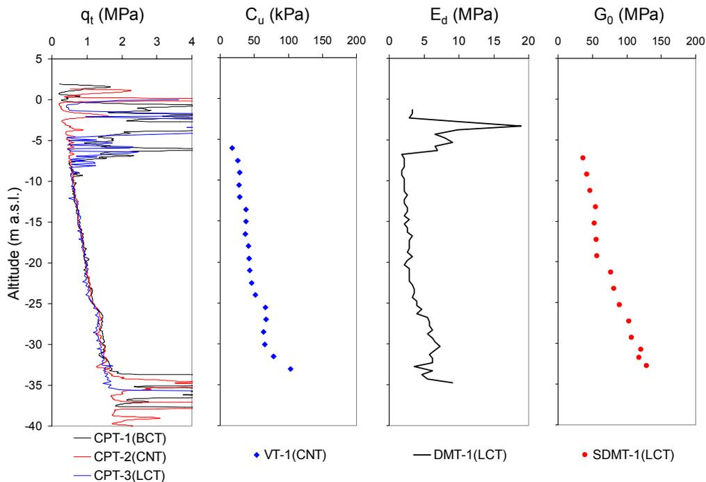
Figure 2. Representative CPTU, VT, DMT/SDMT profiles in Ploče, Croatia.
