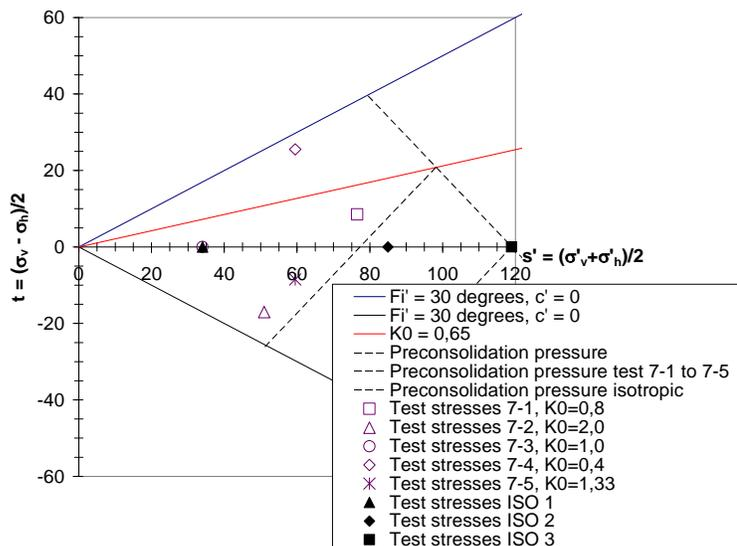
Figure 1. Consolidation stresses for tests 7-1 to 7-4 and ISO1 to ISO3.
