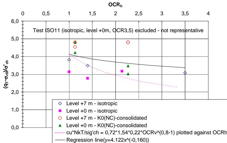
Figure 2. The net cone resistance normalised against the horizontal preconsolidation pressure and plotted against the OCR in the horizontal direction.
