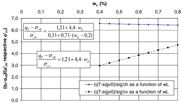
Figure 3. The net cone resistance normalised against the horizontal preconsolidation pressure and the vertical preconsolidation pressure respectively and plotted versus the liquid limit.
