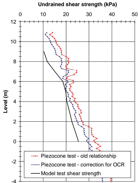
Figure 4. Undrained shear strength calculated from the model piezocone test results compared with calculated field piezocone test results.
