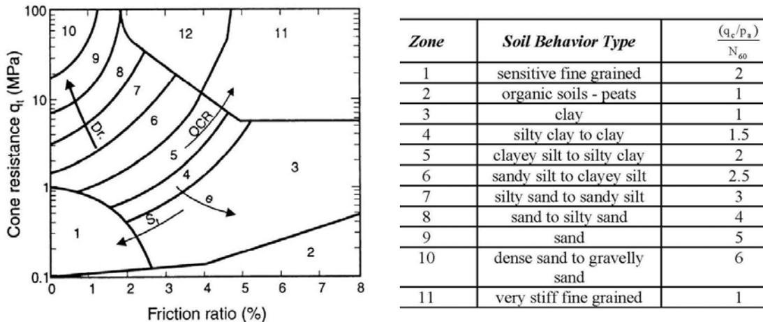
Figure 1. Ratio of normalized cone tip resistance and  $N_{60}$  for different soil behavior types (modified from Robertson et al. 1986)
