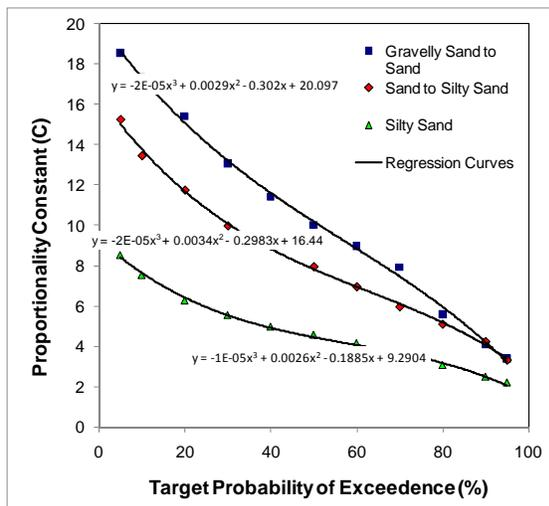
Figure 7. Variation of the proportionality constant ( $C$ ) with the probability that field data will exceed the values predicted using Equation 5.
