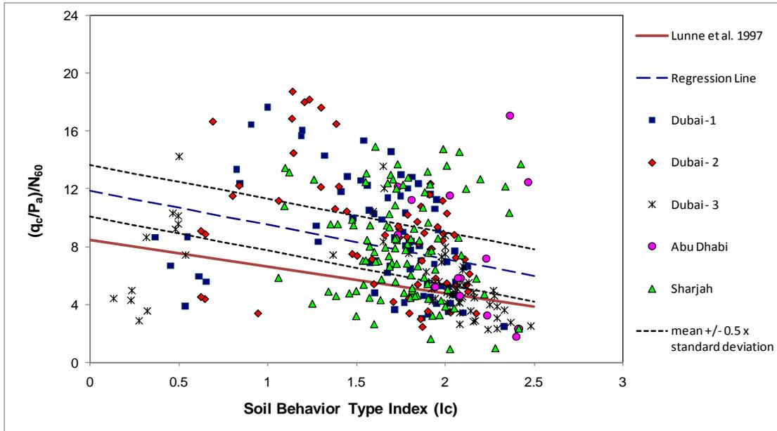
Figure 4. Applicability of the  $I_c$ -based correlations of Lunne et al. (1997) to the UAE calcareous sand.
