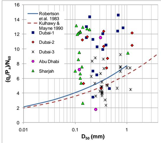
Figure 2. Applicability of the  $D_{50}$ -based correlations of Robertson et al. (1983) and Kulhawy and Mayne (1990) to the UAE calcareous sand.
