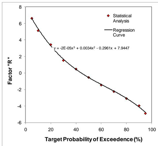
Figure 6. Variation of the factor ( $R$ ) with the probability of that field data will exceed the values predicted using Equation 6.
