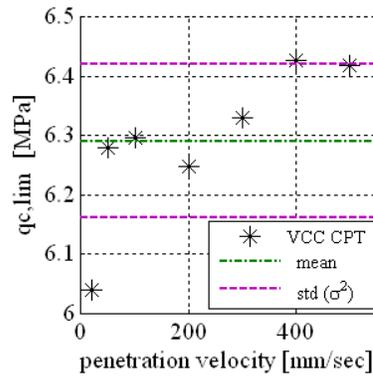
Figure 6. Influence of penetration velocity on cone resistance.
