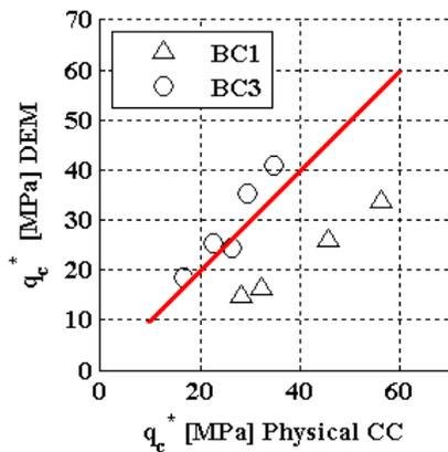
Figure 5. Comparison of corrected cone resistance from DEM VCC CPT (Series II) and physical parallel tests on Ticino sand
