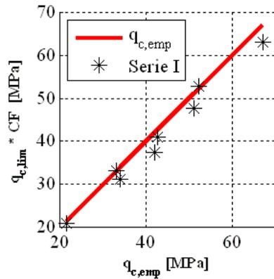
Figure 3. Comparison of corrected cone resistance from isotropically confined DEM tests and the predictions of the empirical correlation obtained for Ticino sand Eq. 4.
