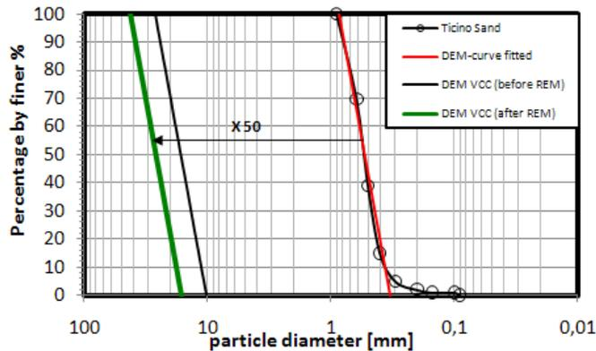
Figure 1. Grain size distribution of Ticino sand and DEM models
