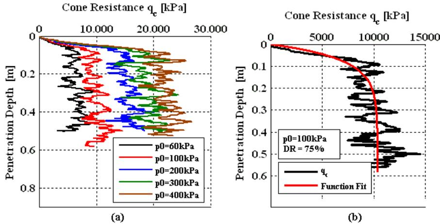
Figure 2. Raw cone penetration resistance curves from test Series I: (a) tests with target  $D_R = 75\%$  and (b) example of curve-fit for the extraction of limit cone resistance, Series I,  $p_0=100\text{kPa}$ ,  $D_R=75\%$ .
