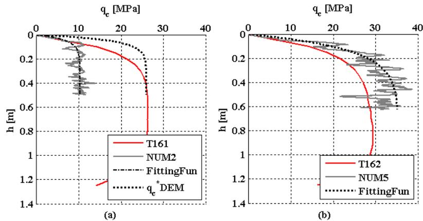
Figure 4. DEM VCC cone penetration curves and physical parallel tests on Ticino sand (a) test T161 BC1 (b) test T162 BC3
