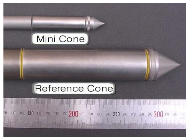
Fig. 1 Comparison between the 2 \text{ cm}^2 and the 10 \text{ cm}^2 cone penetrometers
