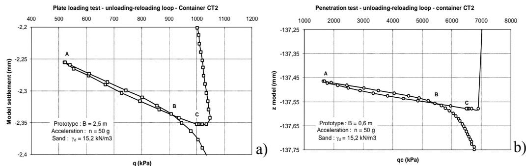
Figure 5. Typical unload-reload loops for (a) plate loading test (b) cone penetration test (CT2)
