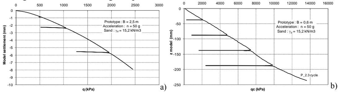
Figure 4. Typical example of (a) plate loading test and (b) cone penetration test profile with unload-reload loop (CT2)
