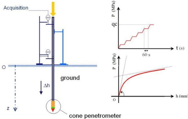
Figure 1. The principle of the cone loading test and the loading program
