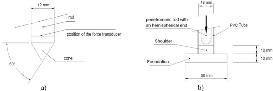
Figure 2. Description of the cone and the plate used in the tests
