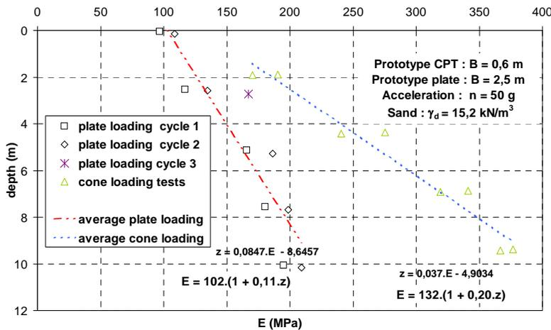
Figure 8. Secant modulus obtained by plate loading test and reloading modulus of cone loading test in centrifuge - Container CT2 ( $\gamma_d = 15.20 \text{ kN/m}^3$ )
