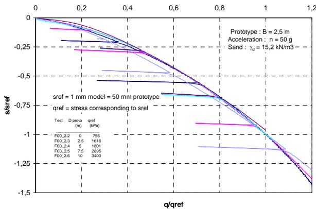
Figure 7. Plate loading tests - Container CT2 ( $\gamma_d = 15.20 \text{ kN/m}^3$ ) – non dimensional curves
