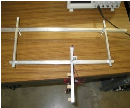
Fig. 3. A model of test frame with bender element
