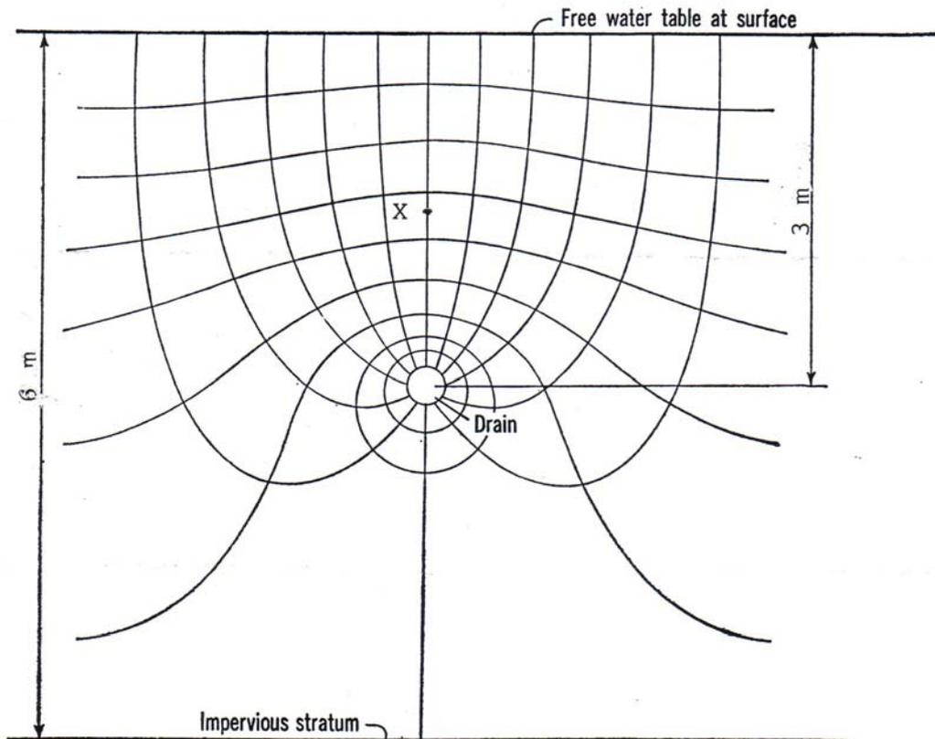
Figure 7.11. Flownet around the Horizontal Drain for Ex. 7.3
