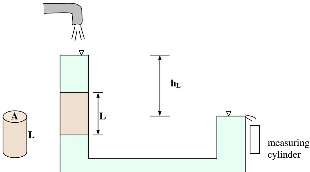
Figure 7.6 Constant head permeability test
