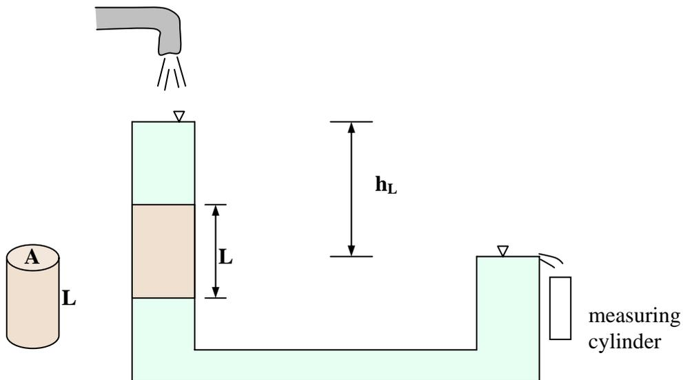
Figure 7.6 Constant head permeability test
