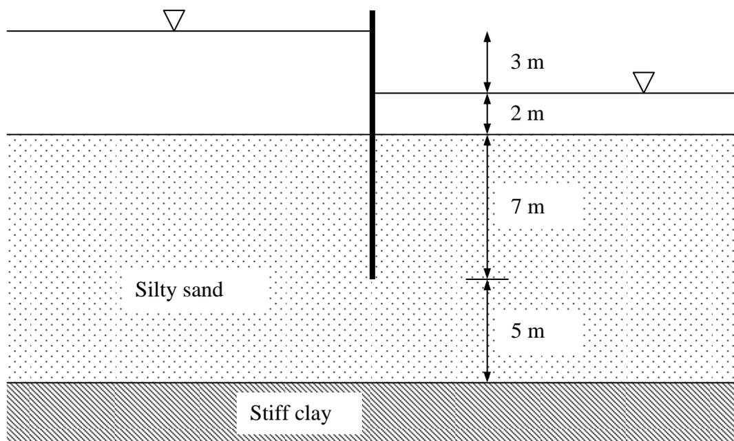
A stiff clay layer underlies a 12 m thick silty sand deposit. A sheet pile is driven into the sand to a depth of 7 m, and the upstream and downstream water levels are as shown in the figure. Permeability of the silty sand is  $8.6 \times 10^{-4} \text{ cm/s}$ . The stiff clay can be assumed to be impervious. The void ratio of the silty sand is 0.72 and the specific gravity of the grains is 2.65.
