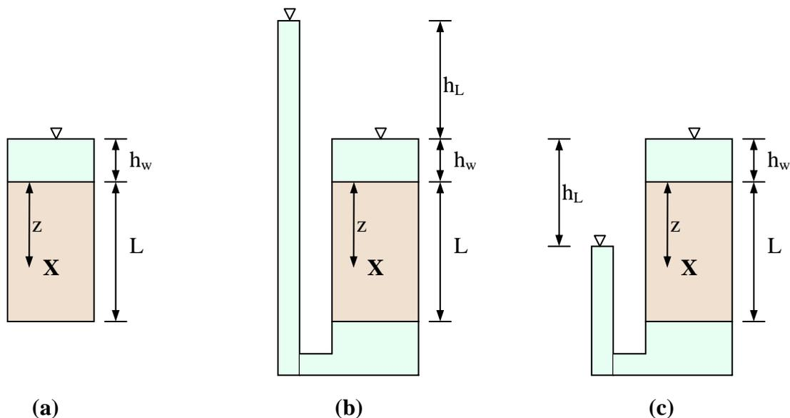
Figure 7.8 Three different scenarios (a) Static (b) Flow-up (c) Flow-down
