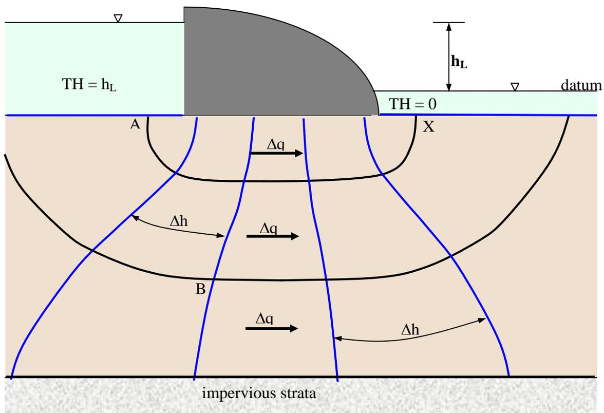
Figure 7.9 Streamlines and equipotential lines
