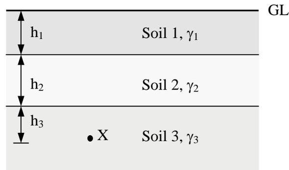
Figure 6.2. Overburden stress at a point in a layered soil
