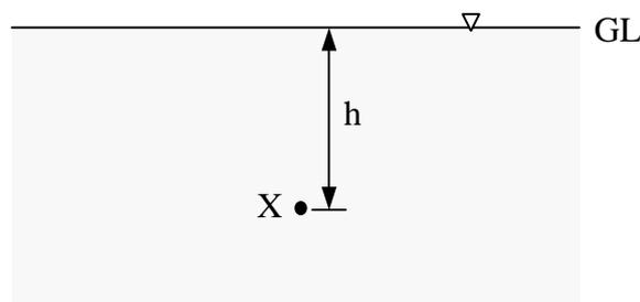
Figure 6.3 Overburden stress at a point in a homogeneous saturated soil
