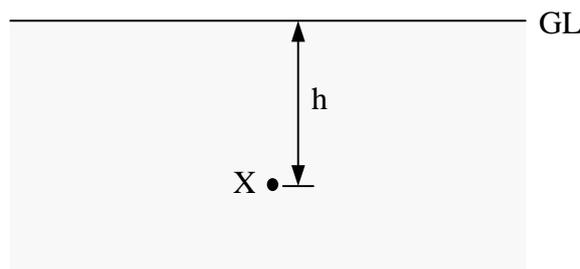
Figure 6.1 Overburden stress at a point in a homogeneous soil
