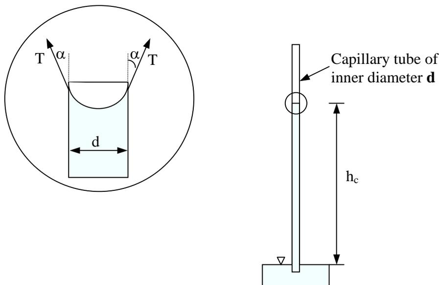
Figure 6.5 Capillary tube in water
