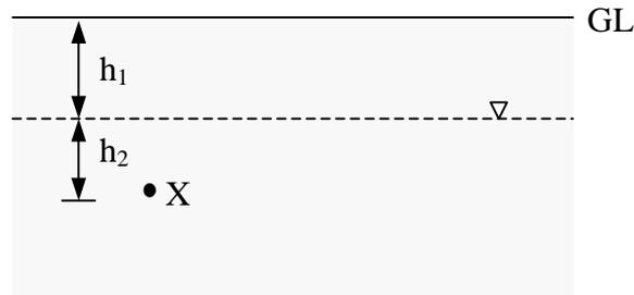
Figure 6.4 Overburden stresses at a point when the water table is below the ground level
