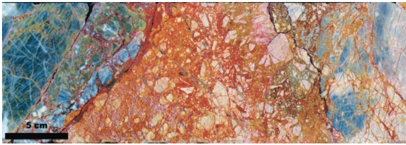
Fig. 7 Transition from blocky rock mass into "bimrock" (central part of picture); mesoscale.
