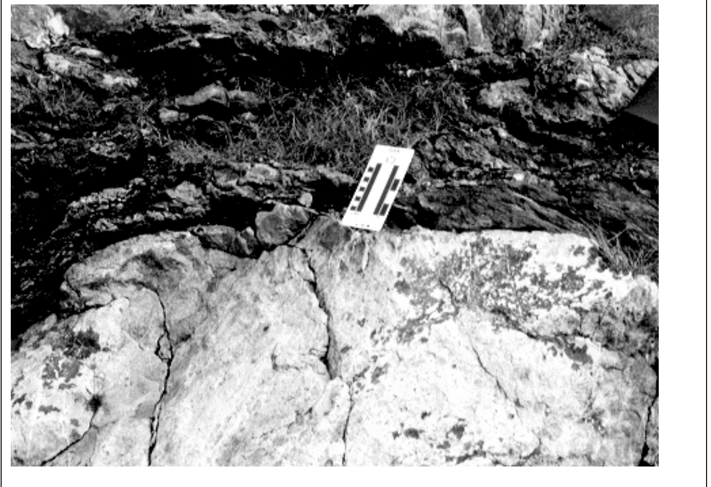
Figure 11. The weakest element in a bimrock is often the block/matrix contact. Gwna Melange, Anglesey, Wales. Photo: E. Medley.
