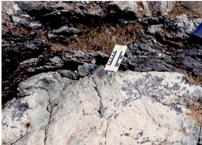
Figure 12. Weakest element in a bimrock is generally the block/matrix contact. Gwna Melange, Anglesey, N. Wales.
