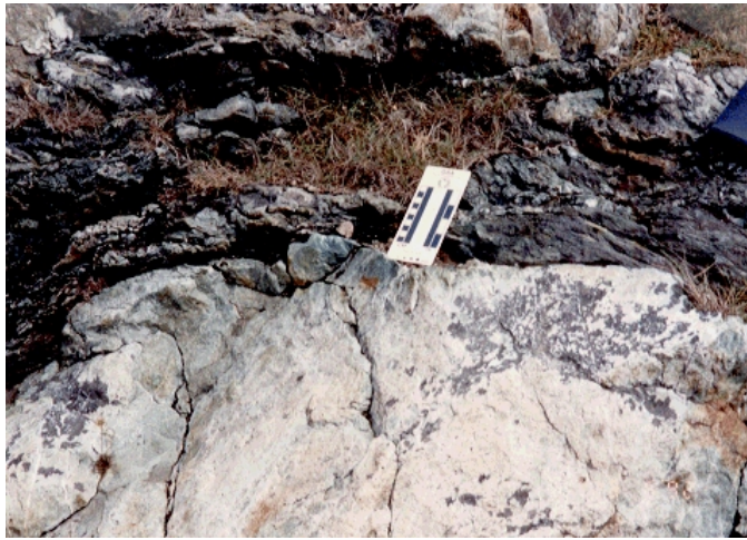
Figure 12. Weakest element in a bimrock is generally the block/matrix contact. Gwna Melange, Anglesey, N. Wales.
