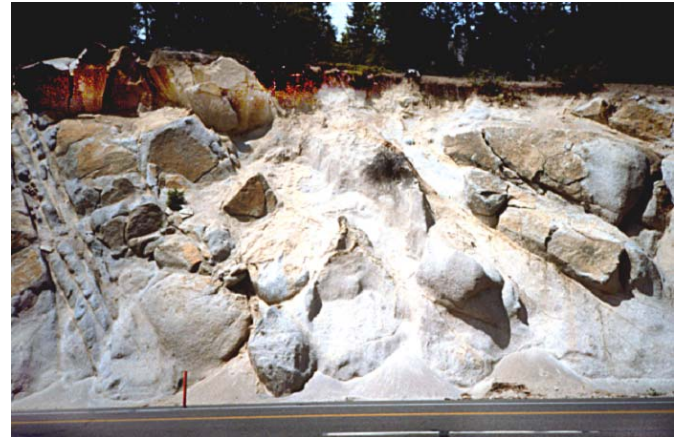
Figure 7. Decomposed granite located in the Sierra Nevada mountains of Northern California. Hard blocks (corestones) surrounded by matrix of “gruss” (granite decomposed to dense sandy soil).
