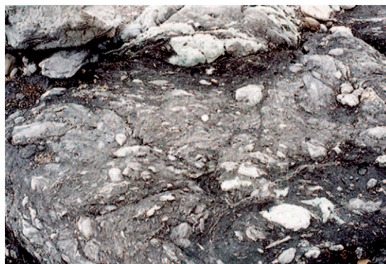
Fig. 1 Typical bimrock outcrop of Franciscan Complex melange near Mendocino, California, USA. The white disk near the center of the photograph is a 2.3 cm diameter coin. (Photo courtesy of Ed Medley, 1994).
