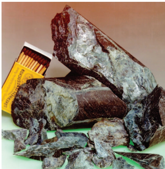
Fig. 3 Drilled core specimen of the Kusan serpentinite.
