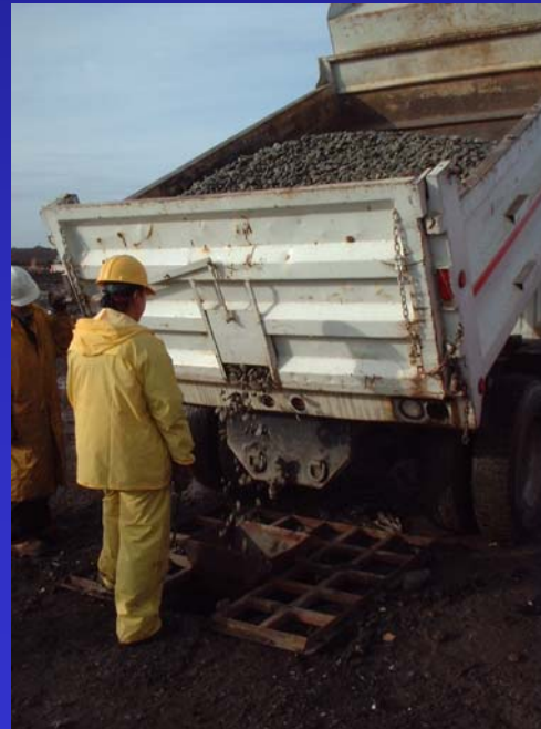
4. Fill with gravel of known unit weight ( V_{waste} )
