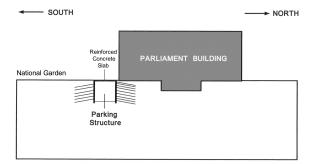
Figure 2. Typical cross section of supported excavation (south side of Parliament building)
