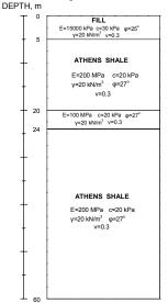
Figure 7. Typical soil profile used in the analyses
