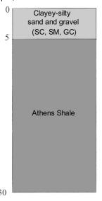
Figure 3. Soil profile at the site of excavation
