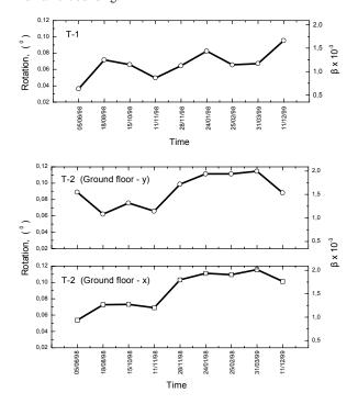
Figure 6. Results of tiltmeters measurements at tilt plates T-1 and T-2
