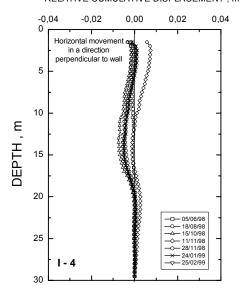
Figure 5. Results of inclinometer measurements at point I-4
