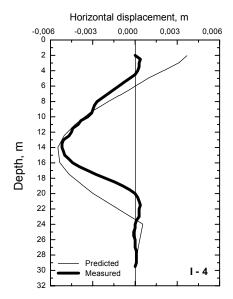
Figure 9. Comparison between measured and predicted horizontal displacements at I-4
