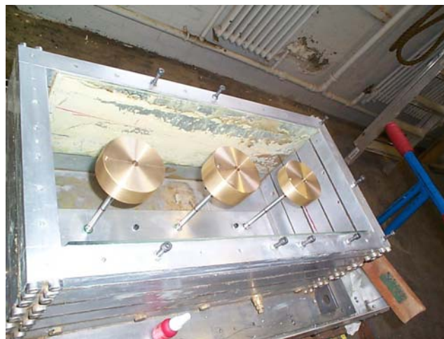
Figure 4.25: The piles and the pile head masses. The piles are fixed at the base. Pile head masses are taken out during sand pouring.
