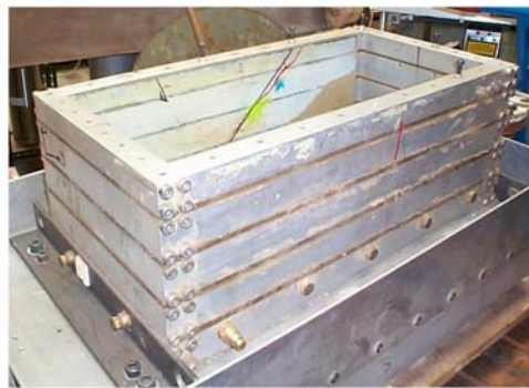
Figure 4.2: ESB box used in the tests.
