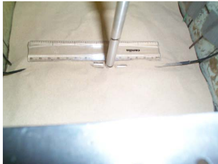
Figure 4.34: PPT's placed in near field of the pile
