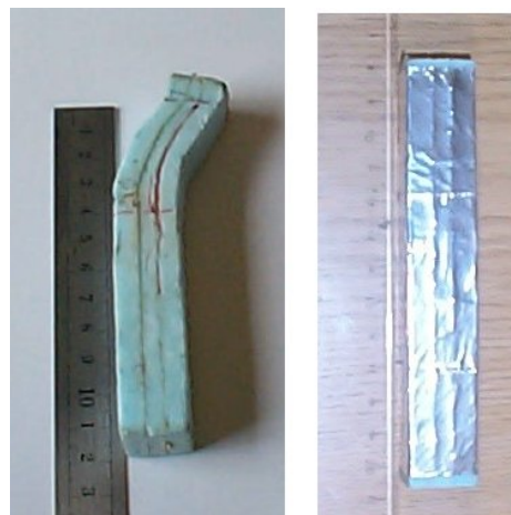
Figure 4.10: Composite pile used in test SB-01.
