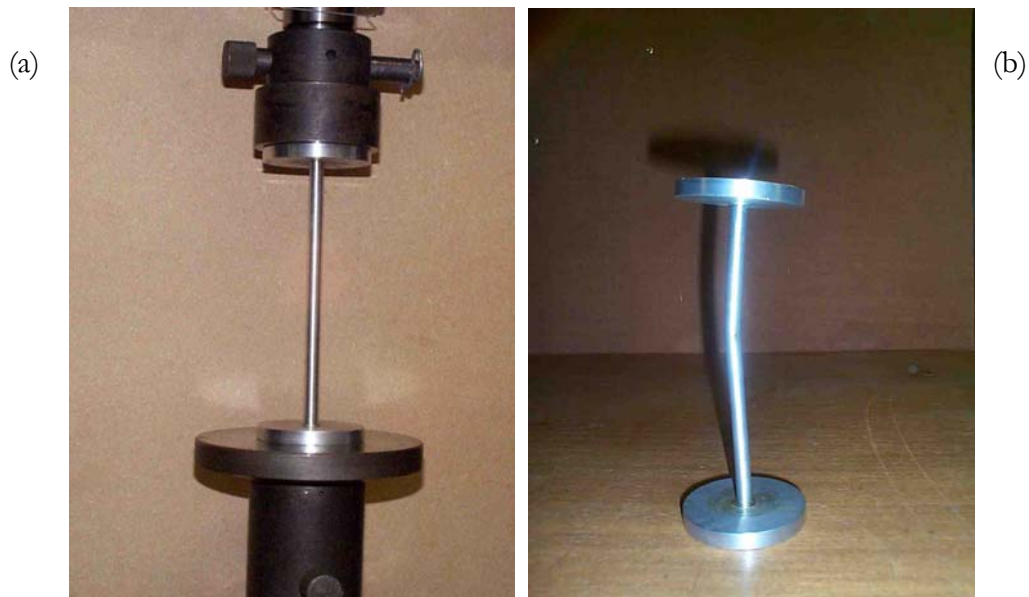
Figure 4.18: Buckling test BT-2; (a): Before the test; (b): After the test.
