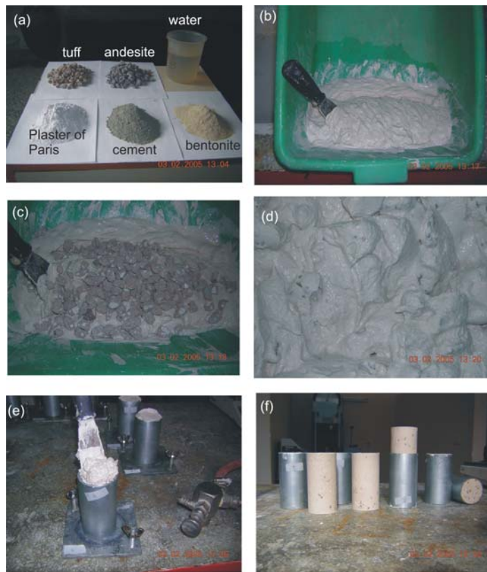
Fig. 2. Preparation stages of the artificial bimrock.
