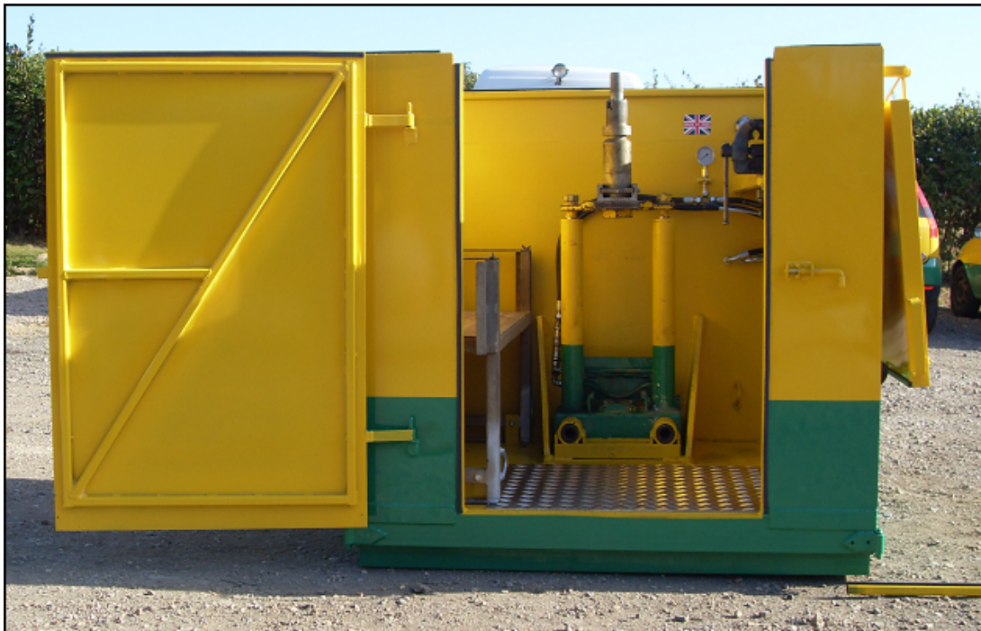
Figure 5. CPT equipment, Lankelma UK 11 (Courtesy Lankelma)
